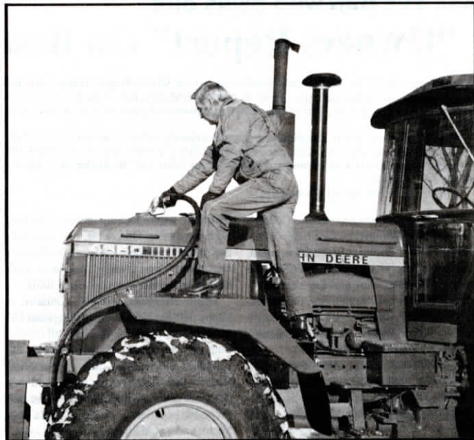
Fenders are built strong enough to serve as refueling step.
