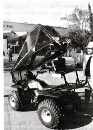
To get on or off, you lift the hinged cab up and forward.
