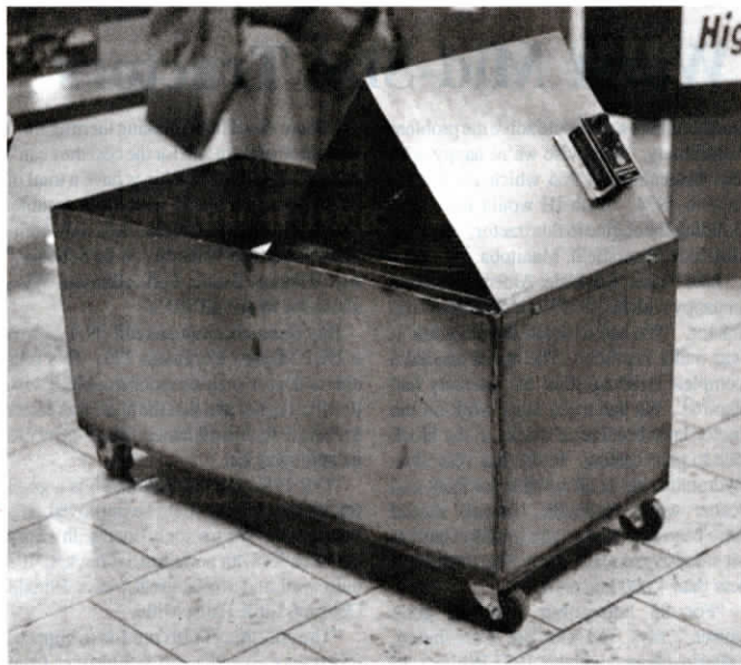
Fan under triangular hood pulls dust-laden air into unit which is half-filled with water.
