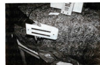
Sensor consists of 5 by 12-in. plastic plate fitted with two stainless steel bars.
