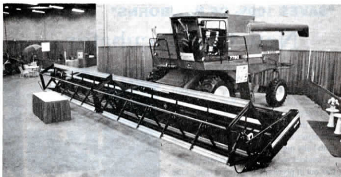
Swather header feeds grain more evenly than a conventional feeder auger, according to the manufacturer. It's also much lighter than a conventional header.
