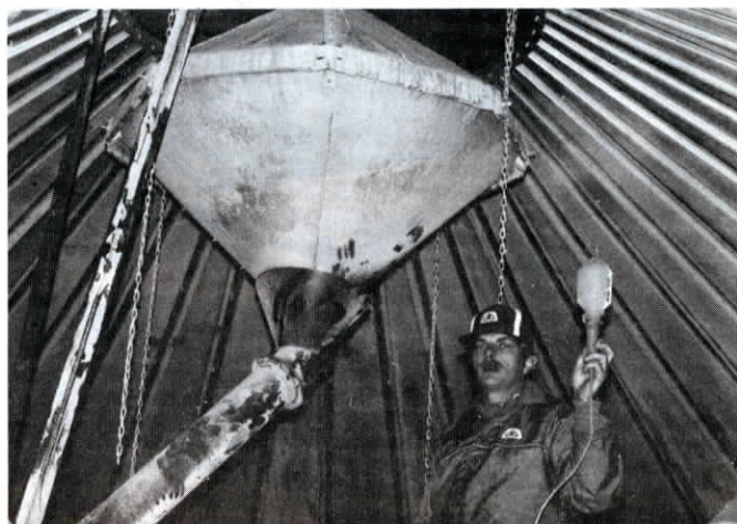
Hoppe stands next to an early prototype of his spreader/cleaner that relied on gravity to clean grain. A pipe at the bottom of the unit carried fines and dirt away.
