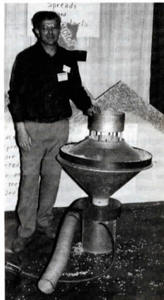
Latest model has a blower/vacuum fan at bottom. Flow of grain is regulated by cylindrical "gate" at top of unit. Flow of grain must be constant over entire spreader to maintain maximum suction power (narrow metal ring on top of screen is there for demonstration purposes only)
