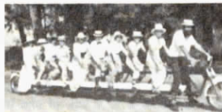
Ten-person bike is 25 ft. long and has a top speed of 20 mph.
