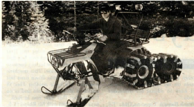
Bolt-on skis and rear track can be removed in minutes.
