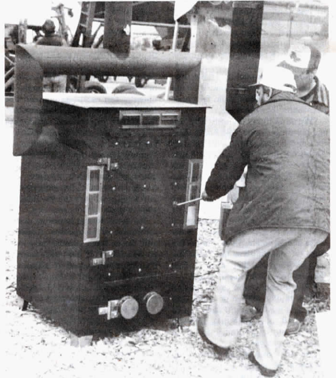
Pipes coming out sides delay flow of smoke and ash for better combustion. Forced feed air flow through center of stove stimulates burning. Inside temperature gets up to 1,200°F.
