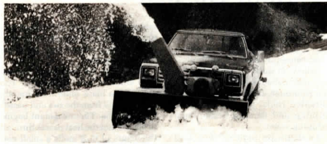
"Snow Mole" motor mounts directly atop blower which can handle drifts up to 3-ft. deep.
