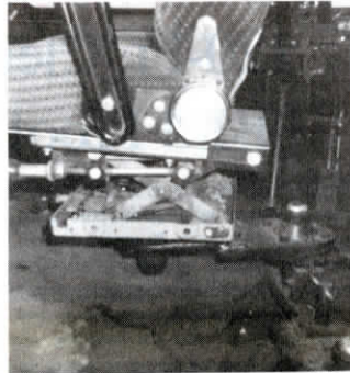
Seat swivels 360°. It attaches to 3 spindles and hubs mounted on offset pivot arms.
