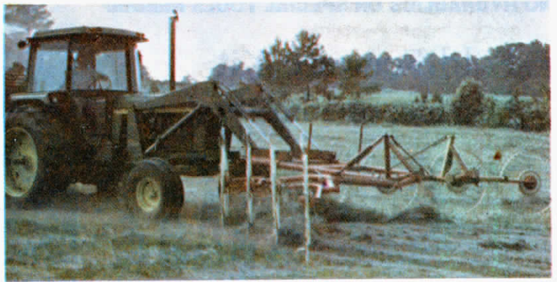
Front-mounted Viccon trapeze rake pulls 18 ft. wide swath into 5 ft. windrow.
