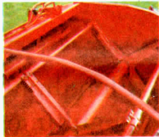
Note that end pipes on 4-bladed rotor are spring loaded. Smaller secondary rotor is on left.
