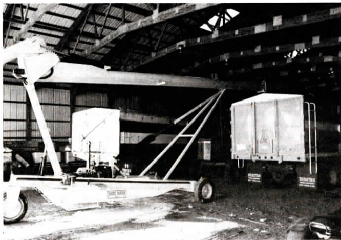
Swing-away intake auger is low enough to fit inside most flat storage buildings. Works great for loading out trucks.
