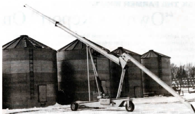
Self-propelled auger can be driven right up to bins. Reaches up to 38 ft. high.
