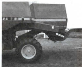
Front end of cteated conveyor rests on combine frame and back end attaches to existing chopper hangers.
