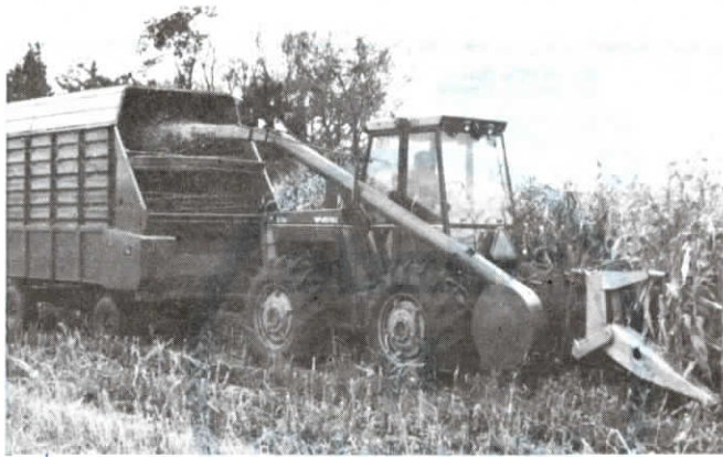
Thor mounted pull-type Deere forage harvester on 3-pt. hitch of his Versatile 276 Bi-Directional tractor. "Visibility and maneuverability are excellent," he says.
