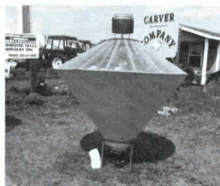
"Spreader-cleaner" has cone-shaped screen positioned above plastic hopper.
