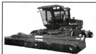
Case-IH 8850 disc mower has 10 oval cutting discs driven by hydraulic motors.
