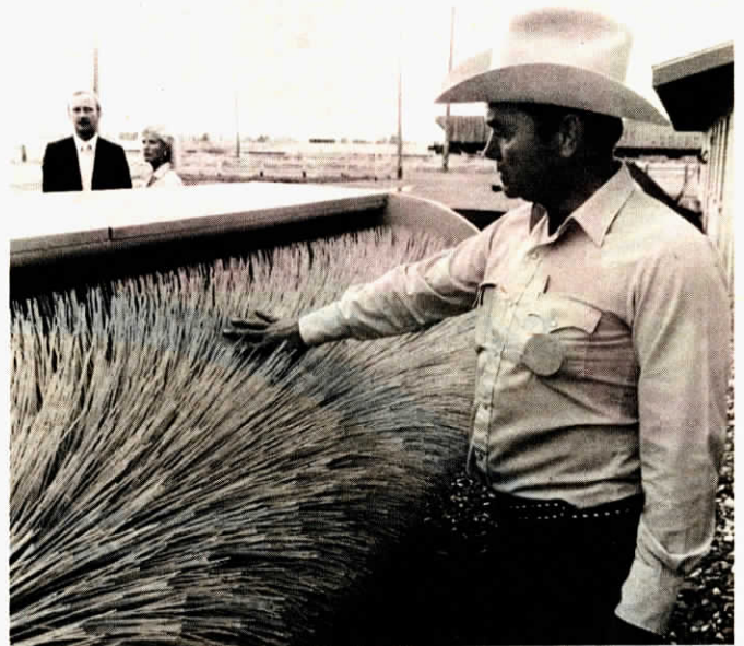
Inventor Ray Anderson with his "Poor Man's Combine" which mounts on self-propelled swather or bi-directional tractor.
