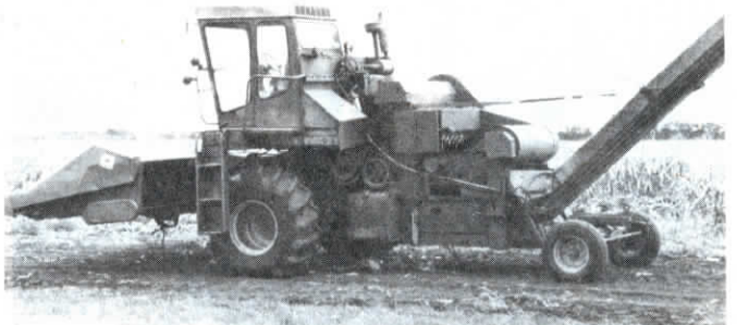
Miller lengthened a 1970 Deere 6600 6-row combine 2 ft. and replaced its threshing system with a New Idea 837 husking bed.
