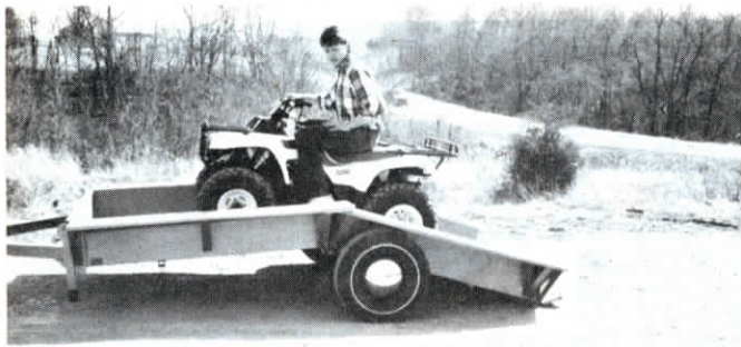
Trailer bed hinges in center, allowing the rear half to drop down as a drive-on ramp.
