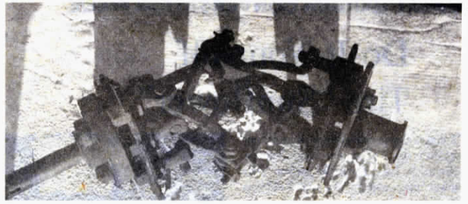
Expandable U-joint, which flexes in either direction, may have been part of the first-ever built-in tractor pto, according to Gilbert Miller.
