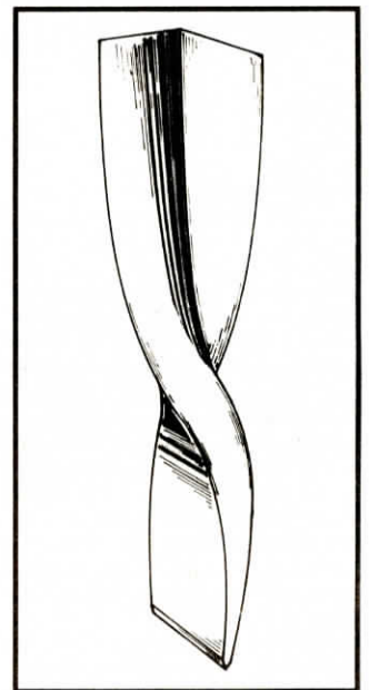
The torquing power of a slight twist helps 7-in. tall wedge split wood.
