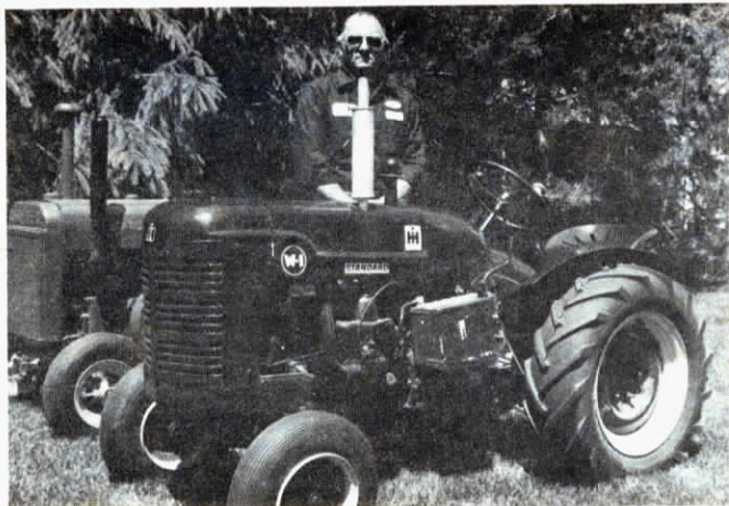
Niemann created this "W-1" half-sized International with parts from a variety of tractors to closely resemble an IH W-4.
