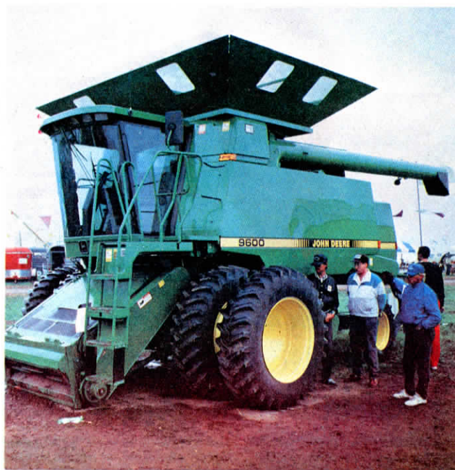
Fold-down bin extension is made out of 12-ga. steel panels fitted with see-through mesh-covered portholes. Short add-on auger mounts inside tank to fill extension.
