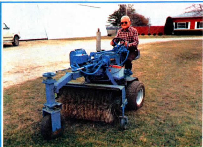
Uhnken built a tractor around a brush originally manufactured for clearing light snows off sidewalks and roadways.
