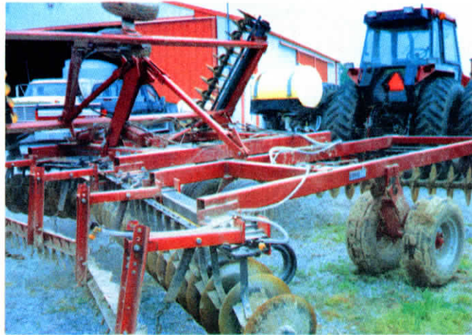
A 30-gal. plastic spray tank is bolted to center section of disk. Note nozzle placement.
