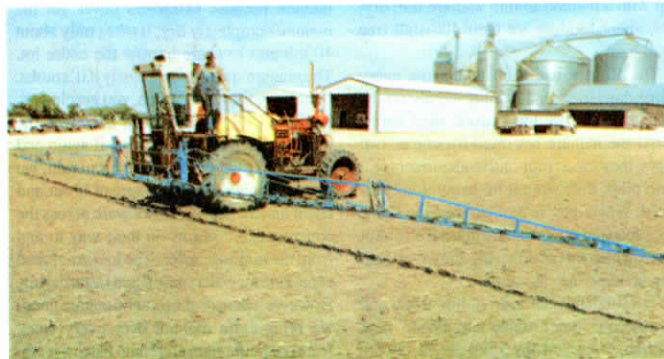
Boom sections are independently-controlled from the cab by solenoid valves. A pair of 3-in. cylinders raises and lowers the boom assembly.
