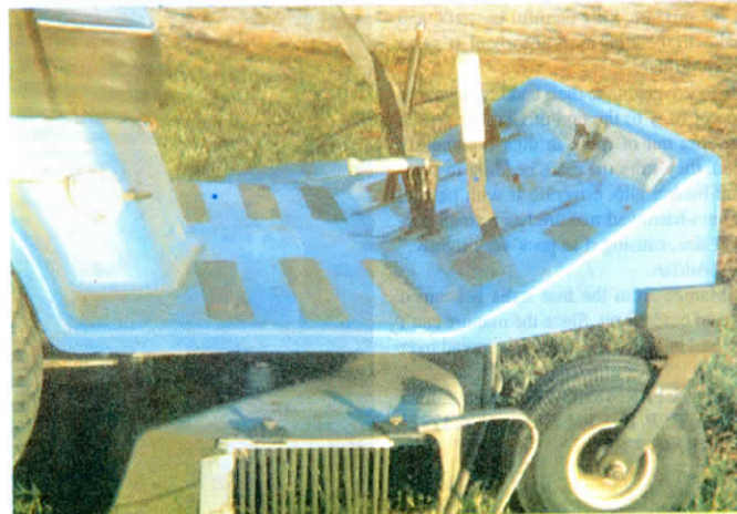
Vertical "fingers" let air blast out but keep leaves in for fine-chop mulching.
