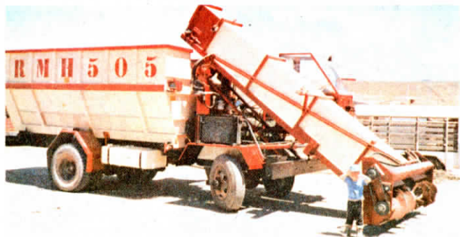
Mixer truck self-loads out of bunk silos, Ag Bags or flat storage with an up-front loader. Each ingredient is precisely weighed as it's loaded.
