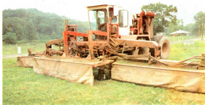
Each of the three separately-powered mower sections floats independently.
