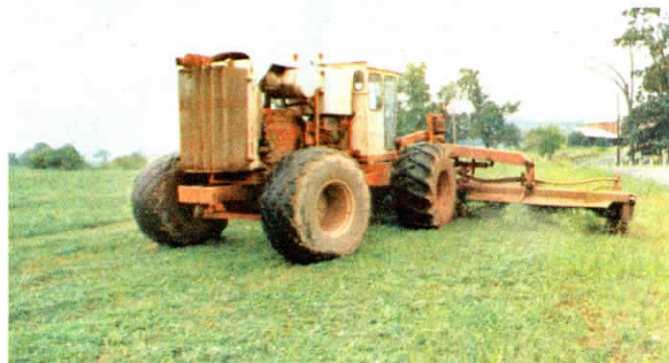
The chassis was salvaged from a self-propelled forage harvester. Air bag shocks let the mower bounce up and over obstructions instead of digging into them.
