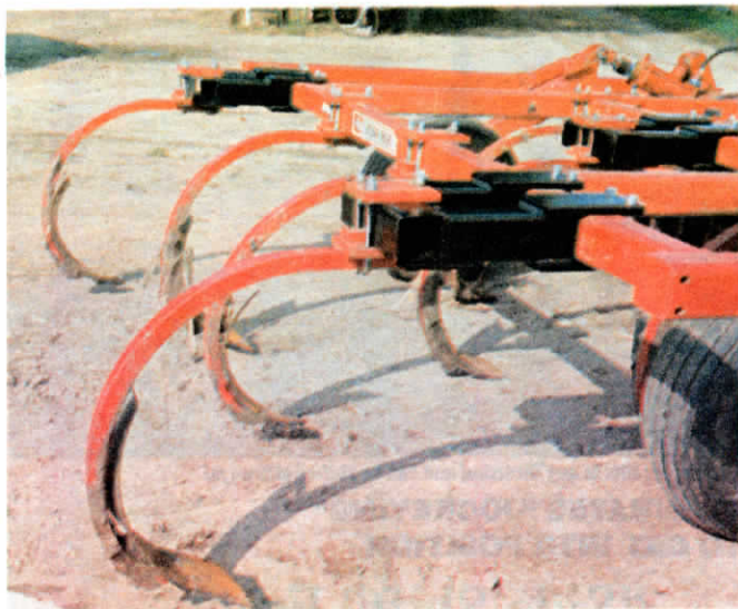
Miller solved plugging problems by converting two rows of shanks into four rows.
