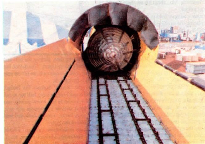
Flighting on spiral bale-chopping cone is fitted with tungsten steel sickle sections.
