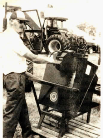
Saw blade is only exposed when operator puts pressure on saw table.
