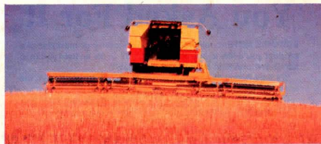
Floating end-sections of 30-ft. head work their way evenly over hilly terrain, boosting combine capacity.
