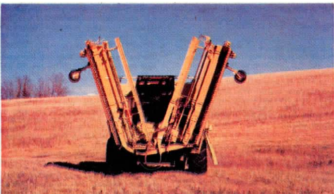
Spring-loaded canvas straps, which act as bats on center 8-ft. section of header, sag loosely out of the way to make room for folding end sections.
