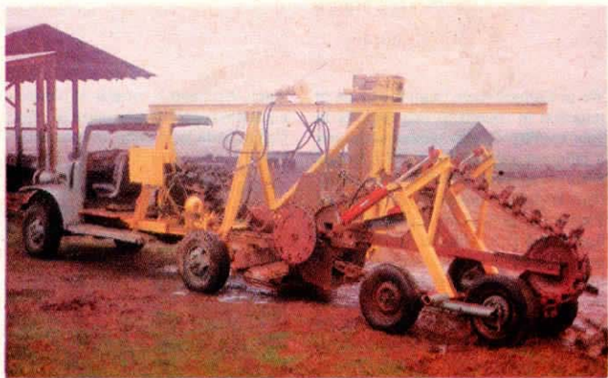
Frank Cawrse Jr. says he can lay up to 250 ft. of tile per hour with his truck-powered tiler.
