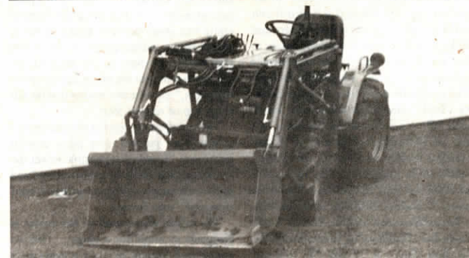
Bucket tilts 5 in. and either side of the bucket moves forward and back up to 15 in.
