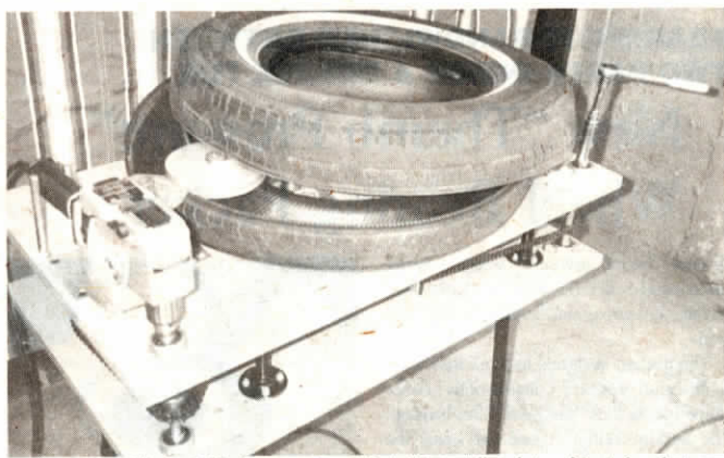
Powered by a 3/4-in. drill, tires can be cut into "donuts" or into wide strips that can then be cut into chunks for easy disposal or burning in wood stoves.
