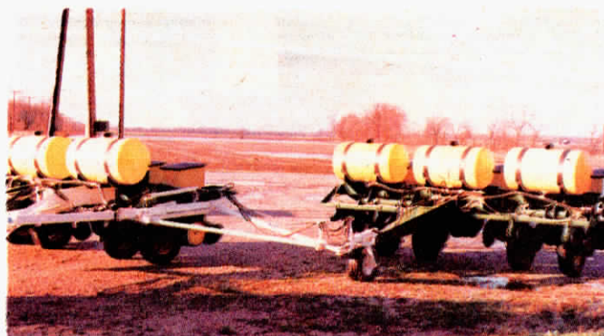
Second planter pivots into position behind front planter for road travel, or for narrow-row planting.
