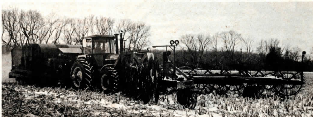
Front-mounted wheel rake pulls stalks and loose ears into a windrow which passes under the tractor.
