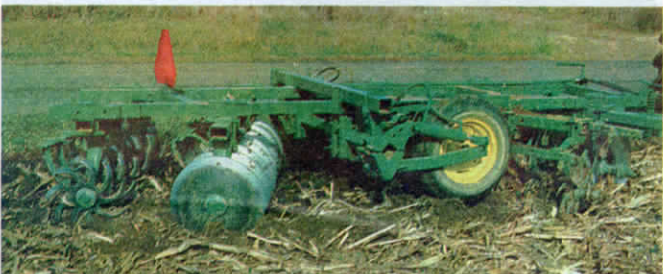
Spider Plow is equipped with two rows of opposite-facing discs, with each gang followed by a row of special-built spider wheels that break up and mix residue.
