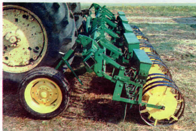
McCoy sows red clover and annual ryegrass between rows of corn using home-built "Betwixt & Between" seeder.
