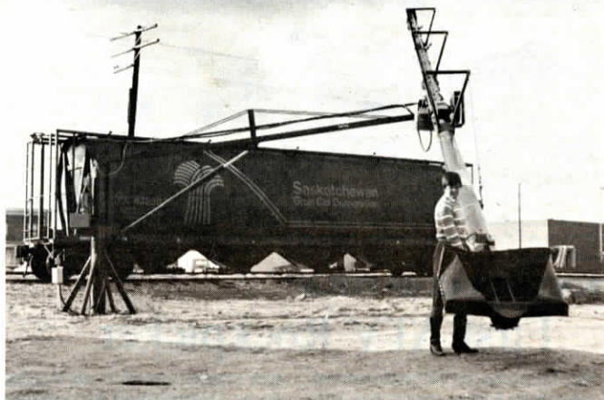
A 10-in., 65-ft. long auger is balanced on a 360° pivoting saddle at the end of a 20-ft. swing arm.
