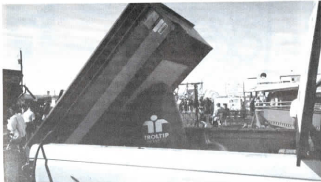
Add-on dump kit makes use of an exhaust-powered bag that lifts up to 1 1/2 tons.
