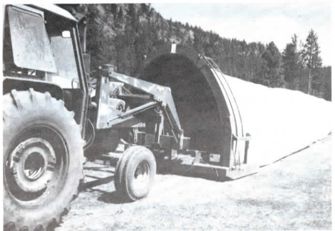
Triangular-shaped bagging frame is fitted with a 200-ft. long "sausage" type bag.
