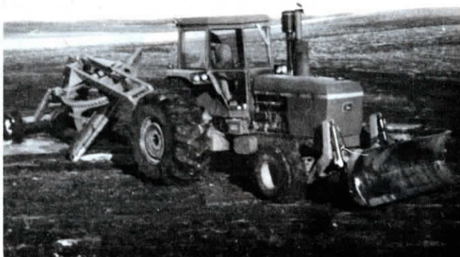
To dig ditches, Isaac mounts a 9-ft. blade on front and a 7-yard scraper on back.
