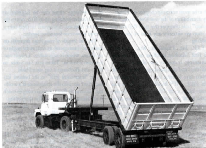
For grain, trailer is equipped with hydraulic dump hoist.
