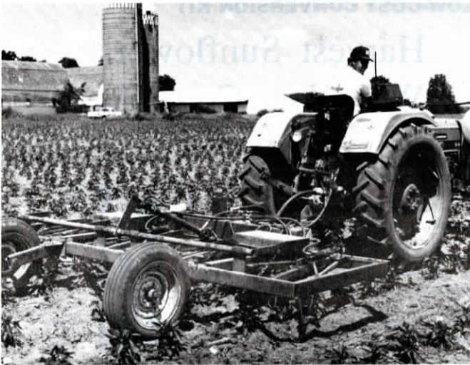
An electric eye triggers hydraulic cylinder above each row that activates shovels.
