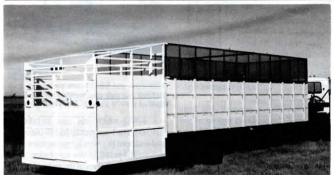
For cattle, trailer is equipped with a “walk on” stock rack attached to rear.
