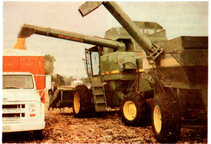
Cart auger has to be far enough back so combine auger can swing unobstructed over front edge of cart and empty into it.
