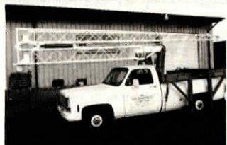
Portable crane can lift up to 5,000 lbs. in the vertical position, above. To transport, right, boom folds down over truck and stabilizer legs fold in hydraulically against the sides.
