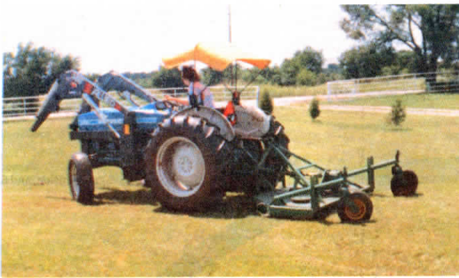
Tractor-pulled mower deck is fitted with heavy caster wheels mounted on brackets that make it easy to adjust height.
