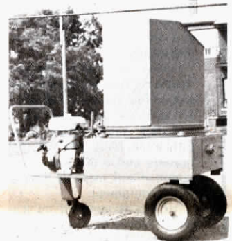
Chop 'N Bed develops enough "rev" to uniformly distribute chopped bedding from front to rear of each stall.
