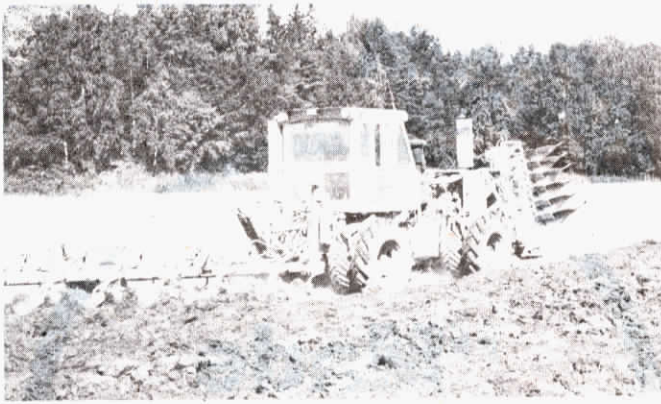
Photo shows original hydrostatic power unit which Soderberg built. Note "left" and "right" hand bottoms mounted front and rear.
