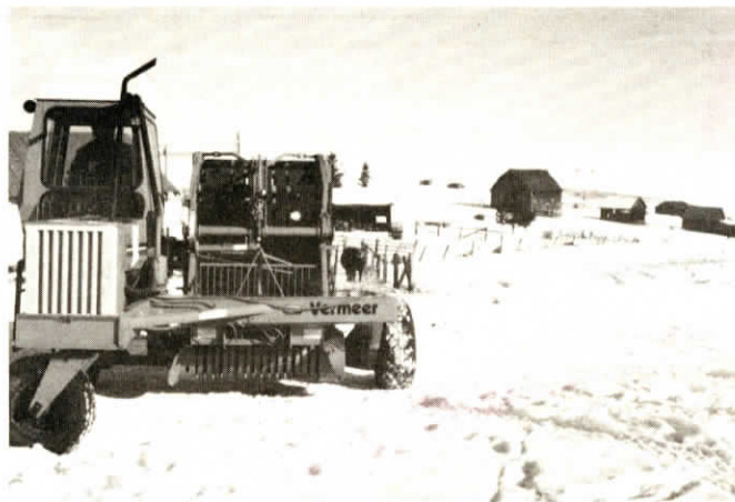
Self-propelled baler makes 360° turns thanks to front caster steering wheel.
