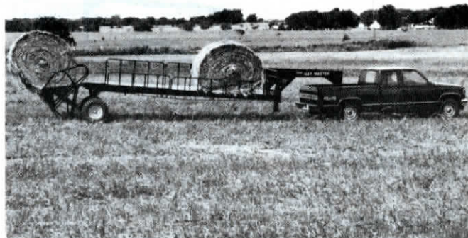
Ground-driven bale lift cradle at the rear lifts the bales onto the trailer's floor.
