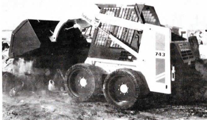
"Big Wheel" tires are fabricated from 3/8 to 1-in. thick sections of used truck tires secured to an oversize rim by steel cable.
