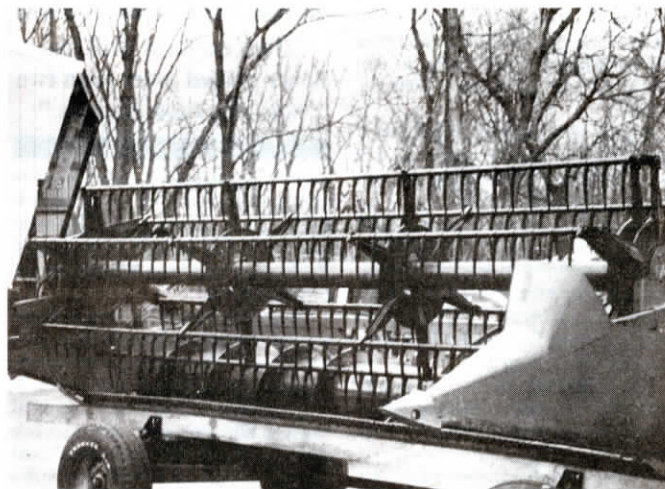
Installation of plastic fingers improves visibility of older wood bat reels.
