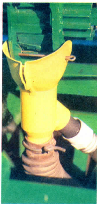
Flow divider's outlet nipple is mounted on side at 45 degree angle. On Deere drills, Smick cuts part of seed cup off and welds flow divider onto bottom.
