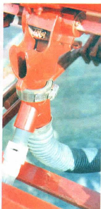
Flow divider's outlet nipple is mounted on side at 45 degree angle. On Deere drills, Smick cuts part of seed cup off and welds flow divider onto bottom.
