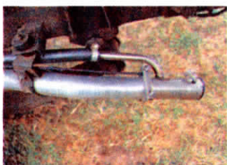
When valve at end of tailpipe is closed, exhaust is diverted to dump bag.
