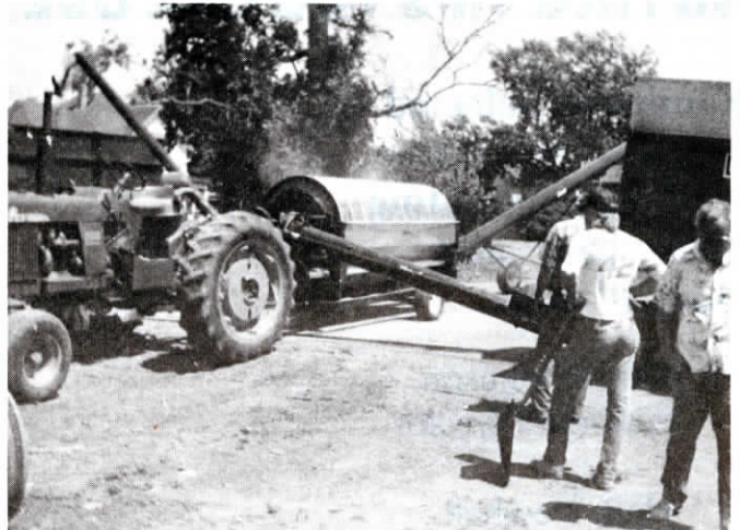
The commercial model, rated at 8,000 bu./hr., has a 48-in. dia. drum.
