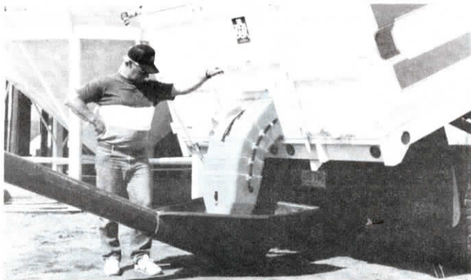
"The Spout" has five all-plastic sections that automatically collapse as box is raised.
