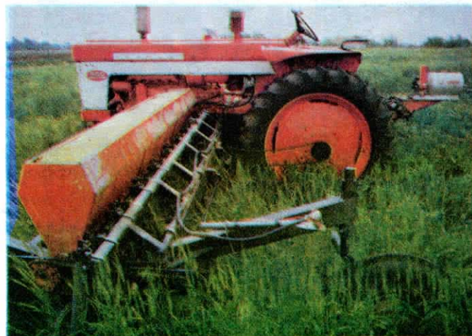
Each drill wing has a "crazy wheel" at outer end for support.
