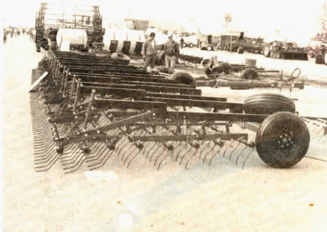
Three rows of slanted teeth at rear pack soil while five rows up front work like conventional harrow.
