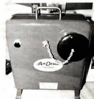
Light or buzzer lets you know if you forget to replace gas cap.
