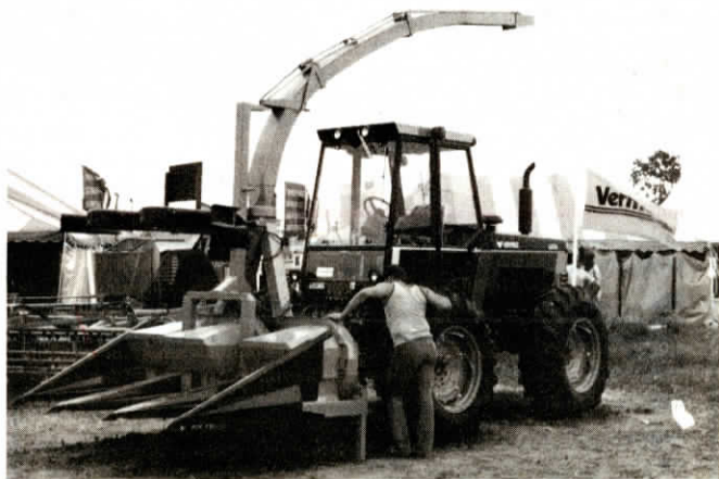
Front-mount Zweeger chopper is shown here mounted on a turned-around Versatile 256.
