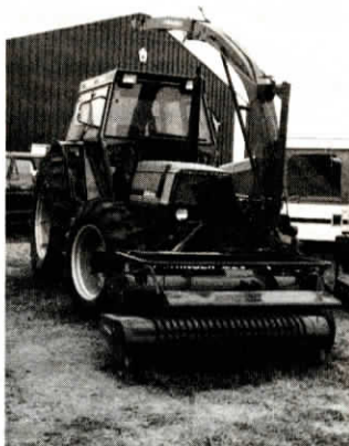
Special features of Pottinger chopper include hydraulic reverser and knife grinder.
