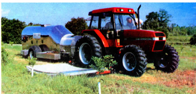
Heated water from 1,500-gal. stainless steel tank is sprayed onto ground through 6-ft. wide side-mounted "boom" that's fitted with ceramic grid.
