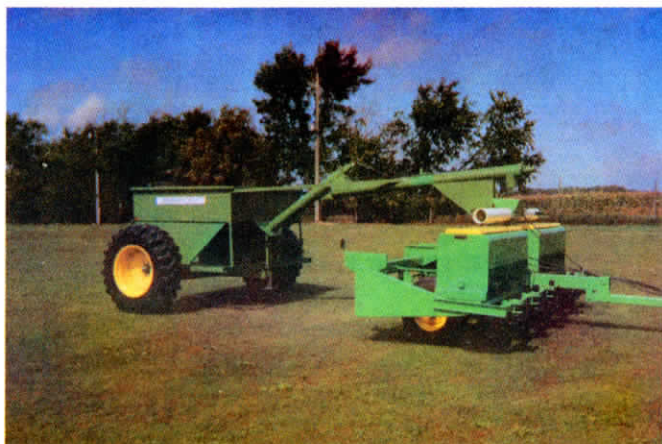
Robinson converts old no-till planters to deep band fertilizer applicators, providing a low-cost way to deep band fertilizer in the fall.
