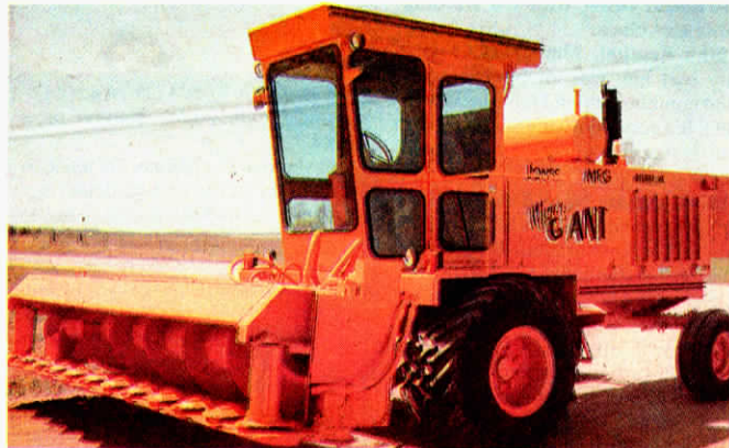
Two Vicon rotary heads were laid end to end to create the 15 ft. long, 12 disc head.
