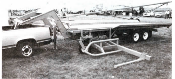
Photos illustrate how axle moves forward to load machinery or unload bales (top) and how axle moves back for transport (bottom).
