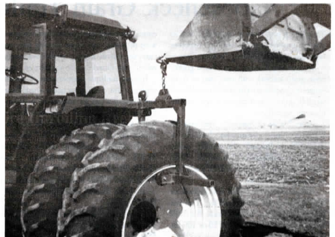
Weight of wheel is on rollers, allowing wheel to spin freely while hanging from front-end loader.
